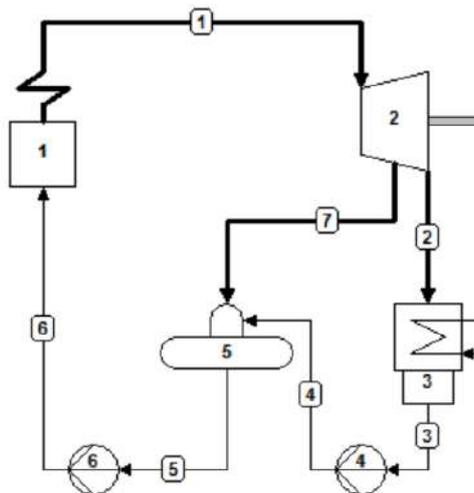
The percentage of bleed steam at 7 required for the open feed water heater is:
